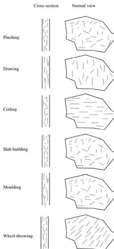
Figure 2: Characteristic features of the main pottery forming techniques (after Carr 1990: fig. 1; Rye 1981).
