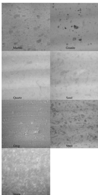
Figure 1: Visibility of different tempering materials. Enhanced radiographic images.
