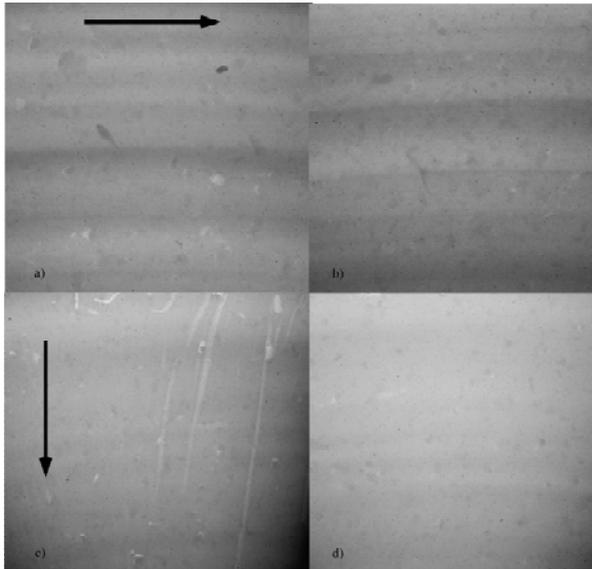
Figure 5: Radiographic features of secondary forming techniques and their lack of impact on primary forming: a) horizontal scraping with a wooden tool can create air pockets, b) no air spaces are visible on the untreated pot; c) vertical knife trimming can leave obvious indentations and air pockets, d) the untreated vessel half. The arrows indicate the direction of the scraping/knife-trimming motion. Enhanced radiographic images.
