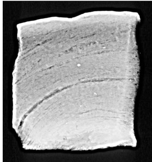
Figure 6: Enhanced radiograph of a Late Minoan saucer fragment from Knossos. Catalogue no 92, Berg 2009. This saucer is wheel-coiled, i.e. it was made of coils which were subsequently shaped on the wheel. The coil seams are clearly visible in the X-ray.
